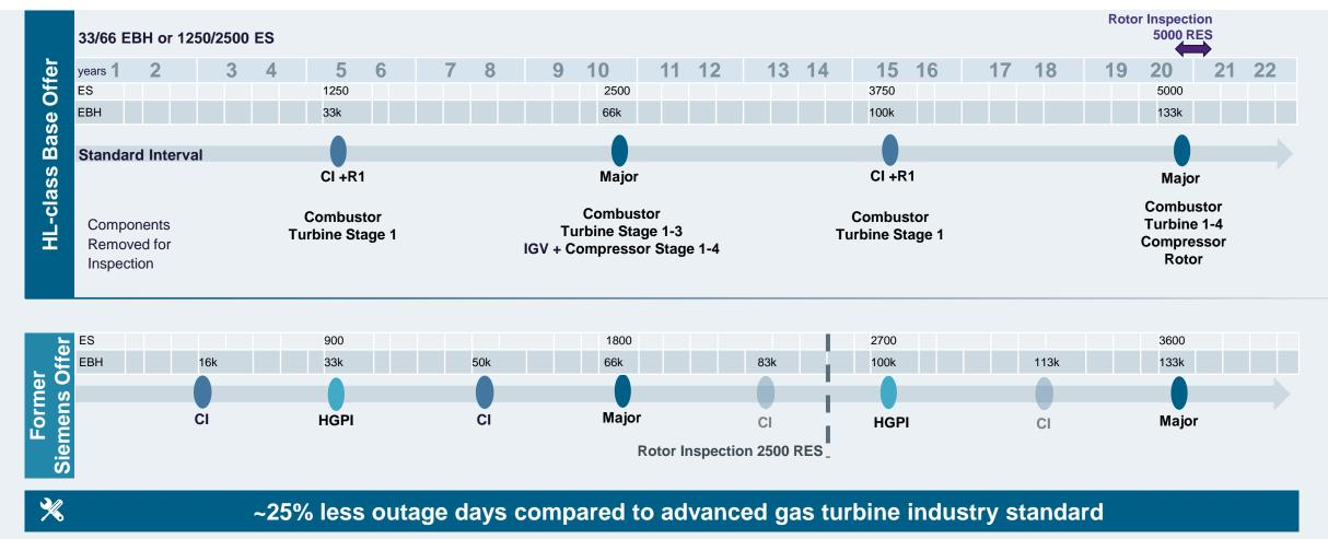
EBH: Equivalent Base Hours, ES: Equivalent Starts, RES: Rotor Equivalent Starts, CI+R1: Combustor inspection w/ Turbine row 1 exchange, Major: Major Overhaul, IGV: Inlet Guide Vane
