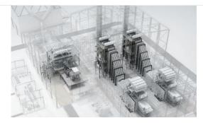
Note: The combined cycle plant SCC-800 is available based on one or multiple SGT-800 gas turbines. Combined cycle performance is based on three pressure non-reheat (3PNRH) bottoming cycle.
